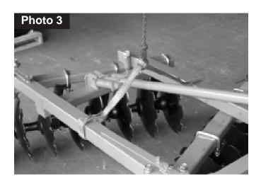
Using a hoist(Photo 3), raise frame approximately 28" off the ground. Loosen the gang beam clamps (ref. #11 & #12) and the gang beam pivot clamps (ref. #9) on front and rear of unit. \*DO NOT REMOVE\* these were pre-assembled on the unit at the factory. Slide gang beam (ref. #8) through gang beam clamp (ref. #11 & #12) and gang beam pivot clamp on front of unit. Repeat the same process on the rear gang beam (ref. #8).
