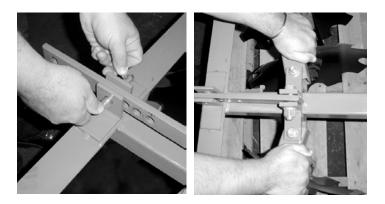
It is important that only one adjustment be made at a time and then tried between each adjustment. Remember each adjustment affects another; therefore, extreme care should be used when adjusting. Each trial run should be made with the tractor in the same gear and approximately the same RPM. Changing discing speed while attempting to adjust will result in excessive time and labor loss due to changing conditions.
