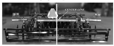
the four 1/2" x 3 1/2" bolts thru the plate welded to the arm. Place the arm mount plate under the tool bar with four 1/2" lock nuts (Photo 37). Check to make sure the roller basket assembly is centered to the disc (Photo 36). Tighten bolts and lock nuts in an alternating pattern to ensure even pressure
