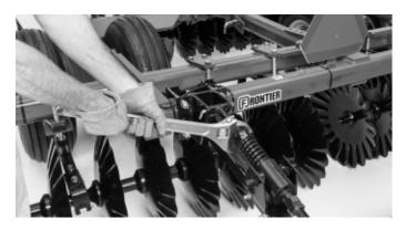
sure the roller basket assembly is level horizontatily with the disc (Photo 40).
