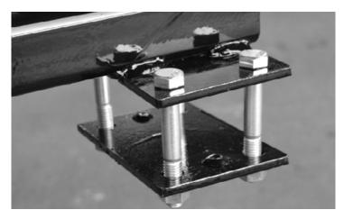
assembly (Photo35). Place roller assembly under arms. Position roller assembly to the center of disc left to right (Photo 36). Remove pin (Photo30, Ref 1) from arm and spring rod assembly. This will let the arms easily lay on top of the tool bar. Place
